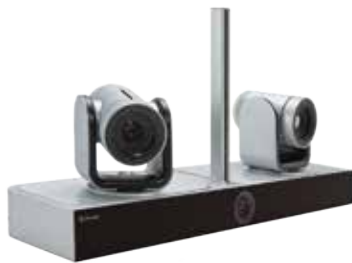
Polycom's EagleEye Director II tracks lecturers as they move around the auditorium
